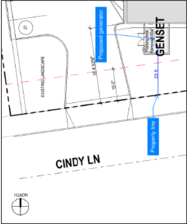
Figure 1 - Generator Site Plan
