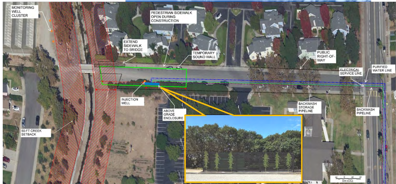
Figure 6. Aerial and Enclosure – IW 1: Meadow View Lane
