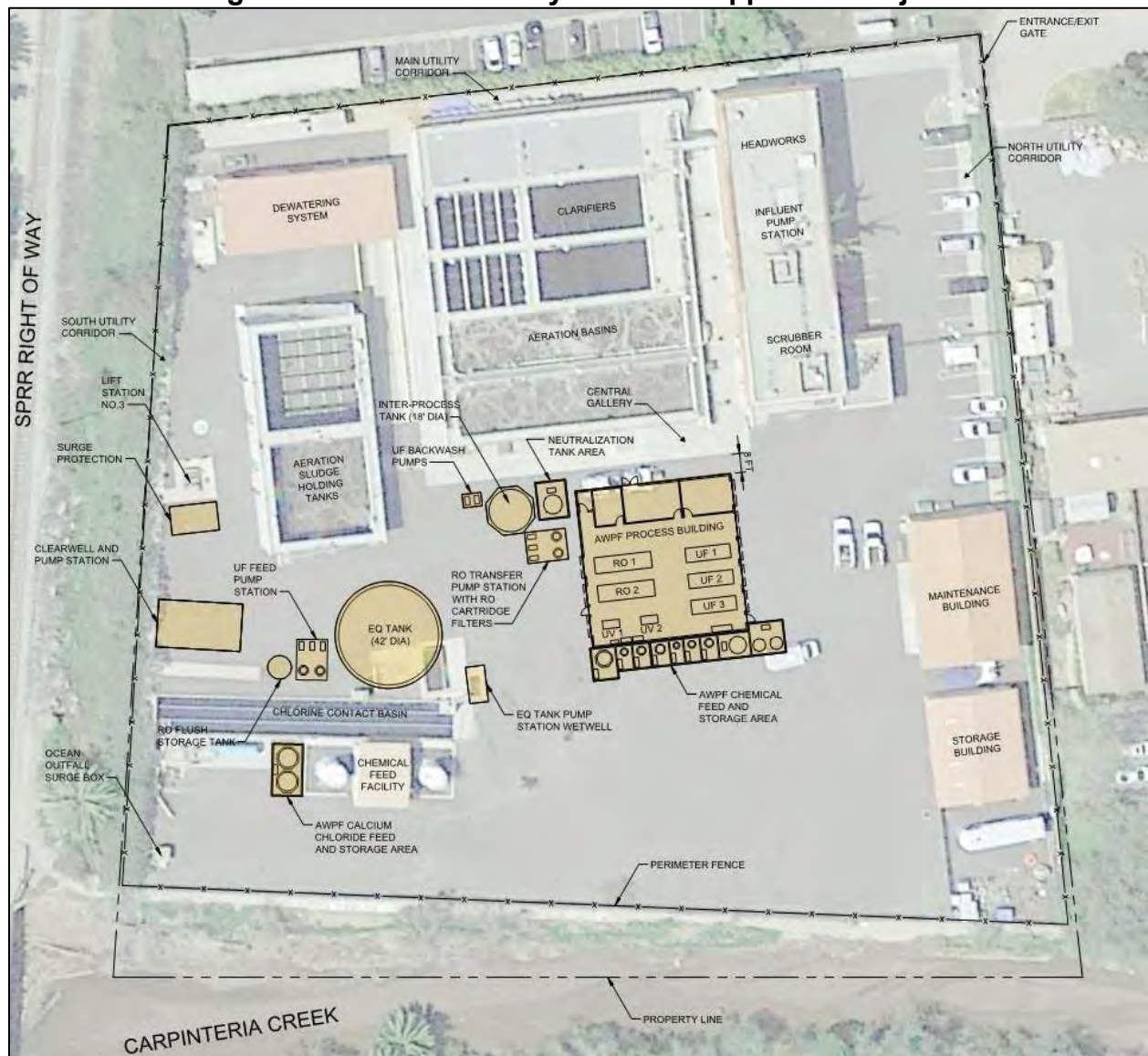
Figure 2-3: AWPf Site Layout under Approved Project
