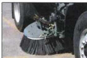
In-cab side broom tilt and extended reach
