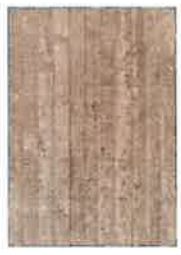
BOARD FORMED CONCRETE WALL
